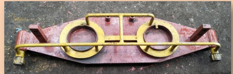
Replacement of LS Beam Ring by Fixture
