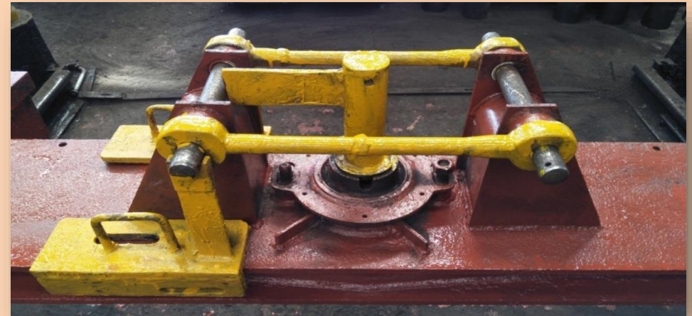
Replacement of Equalizing Stay bkt by Fixture
