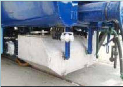
Bio-toilets fitted in coach
