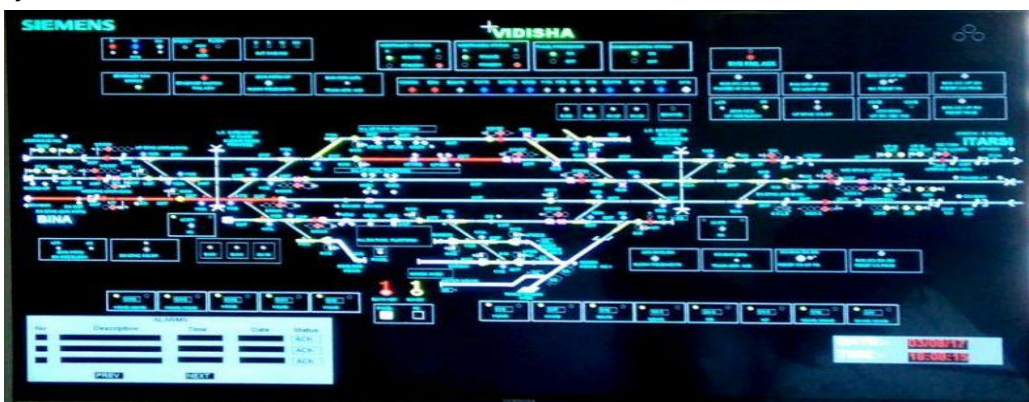
Vidisha Station Visual Display Unit of Electronic interlocking
