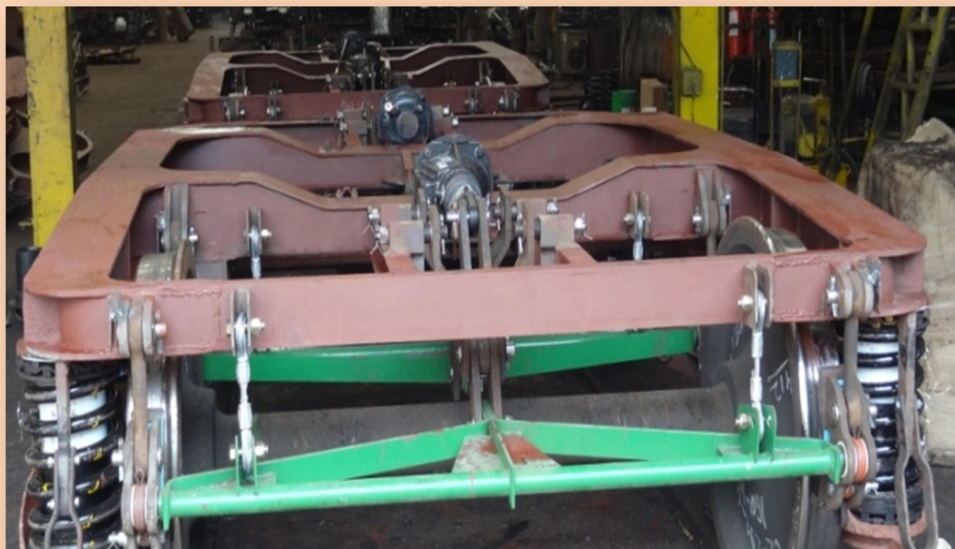
Assembled Bogie for POH Coaches
