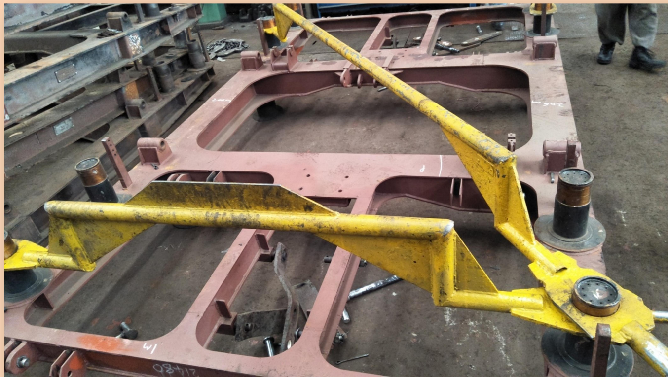
Guide Gauging of Bogie Frame
